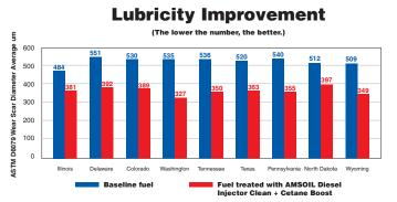
The ASTM D975 diesel fuel standard specifies a wear scar below 520  $\mu$ m in ASTM D6079 testing, while the Engine Manufacturers Association (EMA) specifies a wear scar below 460  $\mu$ m. Testing reveals AMSOIL Diesel Injector Clean + Cetane Boost provides significant lubricity improvement in diesel fuels found across the U.S., delivering improved wear protection. Fuels tested in 2017.
